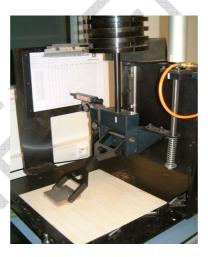
Slip resistance is reported as the static coefficient of friction, a number between 0.00 and 1.00. This number is the average of 4 runs for each formulation.
